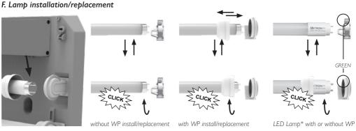
\*By placing the LED lamps, the "AC INPUT" of the lamps, need to be connected in the lampholders with "GREEN" interior.
