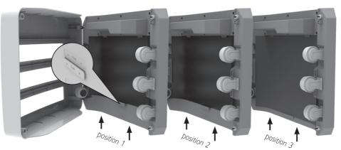
Positions of different glueboards with the position holders. Place the board via bottom side. Push the one of the holders for your board. **Note:** In case of replacement of the lamps use components of the same specifications. Only use genuine spare-parts for service and maintenance.
