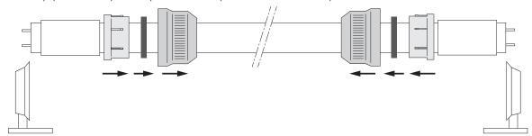
d. Pull the separate parts over the base face from the LED lamp to release them
